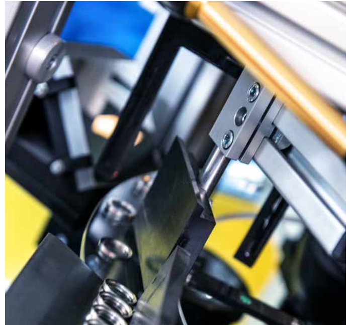
Separating parts with a rotary plate: Dedicated machine concepts by Vester deliver the wanted test results
